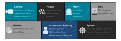
The setup panel includes seven modules. Each module provides some function entries with links for convenient operation.
