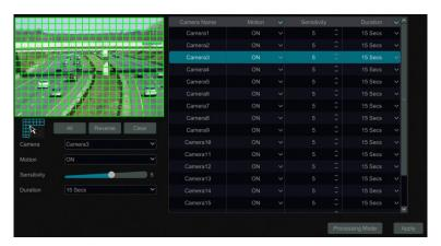
② Select the camera, enable the motion and set the sensitivity and duration of the camera. Sensitivity: the higher the value is, the more sensitive it is to motion. You should adjust the value according to the practical conditions since the sensitivity is influenced by color and time (day or night).
