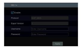
To use this function, the DVR shall be connected to a switch supporting 802.1x protocol. The switch can be considered as an authentication system to identify the device in a local network. If the DVR connected to the network interface of the switch has passed the authentication of the switch, it can be accessed via the local network.
