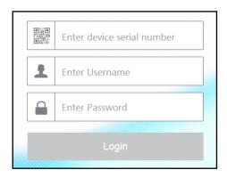
Enter the serial number (click on the tool bar at the bottom of the live view interface to see the serial number of the DVR), user name (the user name of the DVR, *admin* by default) and password of the DVR, select the display language on the top right corner of the interface and then click the "Login" button to go to the web client interface.
