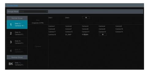
There are four disk groups. By using disk group, you can correspond the camera to disk (the record data of the camera in the group will be stored into the disks in the same group). The DVR with e-SATA interface supports e-SATA recording.
