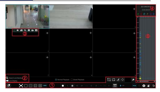
The added cameras will playback their records in the playback interface automatically. You can also add the playback camera manually. Click in the playback window to pop up the "Add Camera" window. Check the cameras in the window and then click "Add" to add playback camera.
