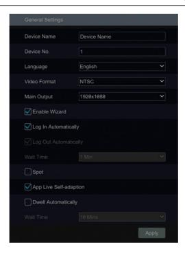
Set the device name, device No., language, video format and main output resolution. Enable or disable wizard, "Log In Automatically", "Log Out Automatically" (if checked, you can set the wait time) "App Live Self-Adaption" and "Dwell Automatically" (if checked, you can set the wait time). Click "Apply" to save the settings.
