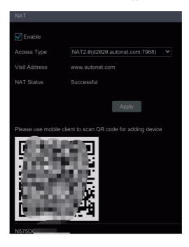
You can scan the QRCode through mobile APP which is installed in the mobile phone or tablet PC to quickly add the device to the server list of the mobile APP.
