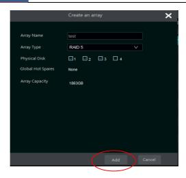
e. Select a hot spare. In the physical disk interface, select the disk that is not in the array and click as shown in the following pictures.
