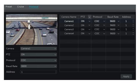
Select the camera and enable PTZ and then set the protocol, baud rate and address of the dome according to the settings of the dome.
