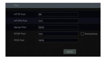
*HTTP Port*: the default HTTP port of the DVR is 80. The port number can be changed to others like 81. The port is mainly used to client remote access. If you want to access the DVR through a web browser, you should enter IP address plus HTTP port in the address bar like http://192.168.11.61:81.
