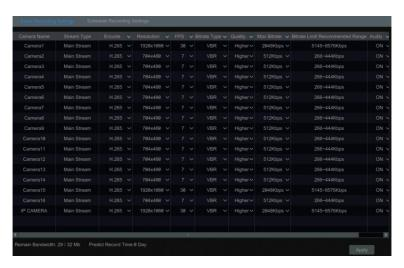
Click Start→Settings→Record→Stream Settings to go to "Sub Stream" interface. Set the encode, resolution, FPS, bitrate type, quality and max bitrate of sub-stream for each camera in the interface and then click "Apply" to save the settings.
