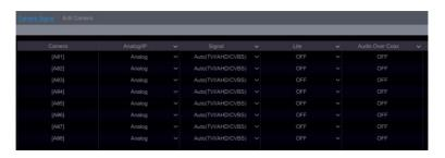
**Note:** You can enable "Lite" in the interface if the DVR supports "Lite" recording. It will lower the recording resolution and increase the recording frame rate. Please enable or disable the Lite as needed.
