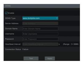
Check "Enable" and then select the DDNS type. Enter the server address, domain name, username and password according to the selected DDNS type. Click "Test" to test the effectiveness of the input information. Click "Apply" to save the settings. After that, the successful connection status can be viewed.
