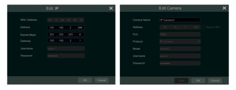
Click to edit the added camera as shown on the above right. Enter the new camera name, IP address, port, username and the password of the camera. You can check "Sync to IPC" to modify the IP address of the IPC via different network segments for being in the same network segment with the DVR. You can click "Test" to test the effectiveness of the input information. Click "OK" to save the settings. You can change the camera name only if it's an analog camera
