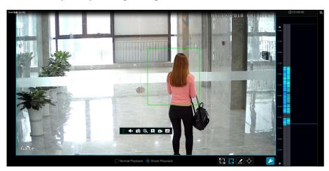
Click and draw a rectangle in the desired area. Then the system will automatically search the record files of this area. The cyan blocks indicate that there are intelligent recording files. Move the cursor to such block and click to play the record.
