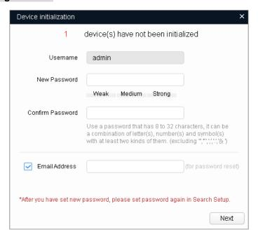
Figure 3-11 Step 5 Set the initialization parameters for the device. See Table 3-4.
