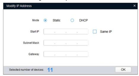
Step 3 Select **Static** mode, and then enter start IP, subnet mask, and gateway.
