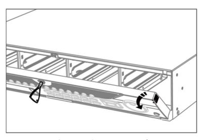
**Figure 1-5 Open Front Panel**
