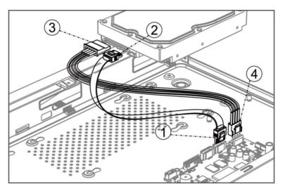
**Figure 1-8 Connect Cables**
