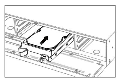
Figure 1-6 Insert HDD
