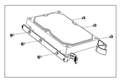
Figure 1-4 Fix Mounting Ears to HDD
