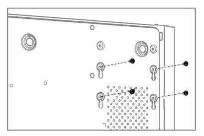
Figure 1-9 Fix HDD to Device Bottom
