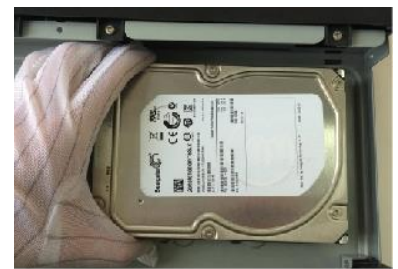
3. Put the HDD into the Device.
