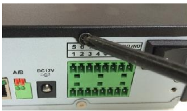
1. Remove the screws on the cover.
