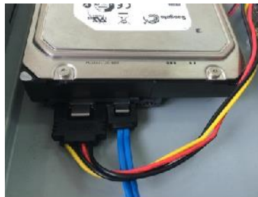
5. Use the HDD cable and power cable to connect HDD and mainboard.
