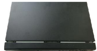
6. Put back the cover and fix the screws.
