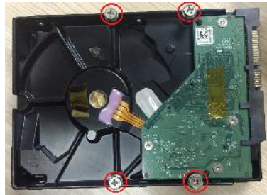
2. Fix the screws onto the HDD, but do not be fastened.
