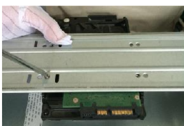
2. Use the screws to fix the HDD onto the bracket.
