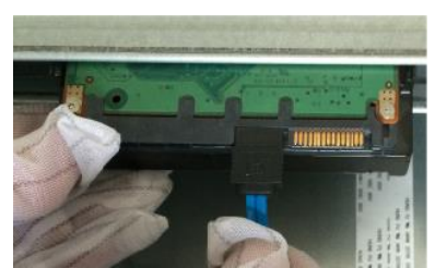
3. Connect one end of HDD cable to the HDD.
