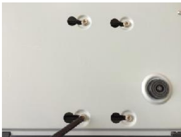
4. Turn the device to see the back side of it. Align the screws of the HDD with the holes on the back of the device, and then fix the screws.
