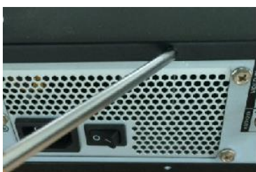
1. Remove the screws on cover.
