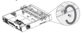
Step 4 Match the four screw holes on the HDD with the four holes on the bracket and then fasten the screws. The HDD is fixed to the bracket.
