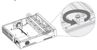
Step 4 Align the four screw holes on the disk to those on the drive bracket and fix the disk on the bracket.
