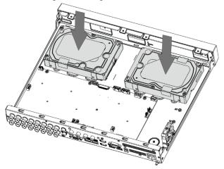
Step 4 Turn the device and put in the other two screws, and then fasten all screws to fix the HDD to the device.
