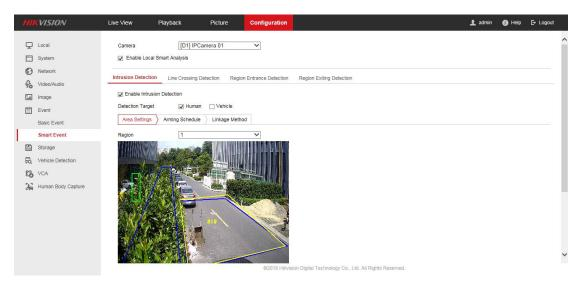
If you don't tick 'Enable Local Smart Analysis', NVR would receive the alarm picture from IPC to filter false alarm(IPC must have the ability to upload alarm picture to NVR).
