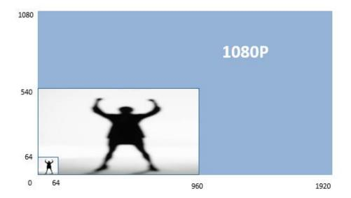
For example, the target in picture below is too large to detect, the man almost covers the whole scene. We suggest adjusting the angle higher so that IP camera can start detecing from a longer distance.
