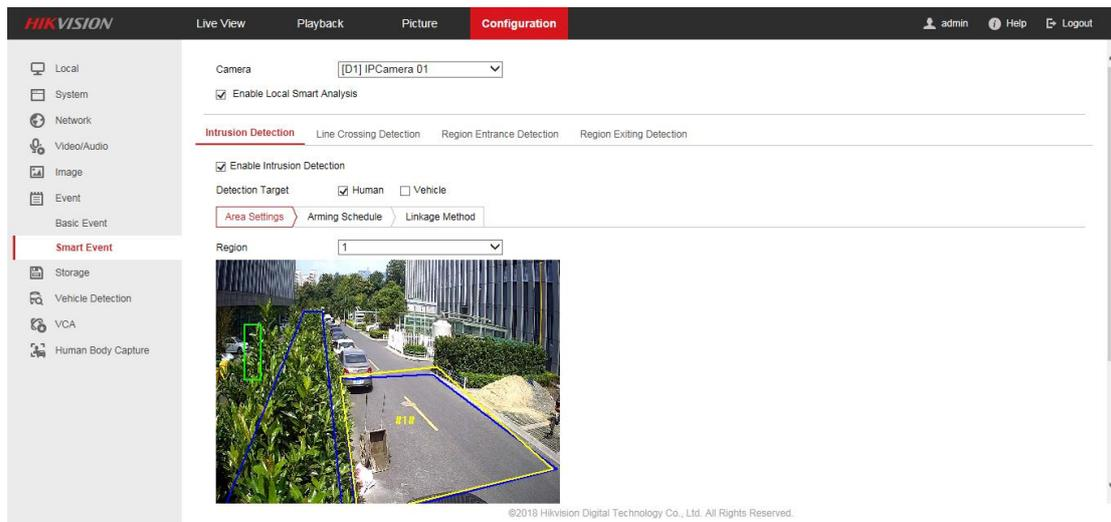
If you don't tick **'Enable Local Smart Analysis'**, NVR would receive the alarm picture from IPC to filter false alarm (IPC must have the ability to upload alarm picture to NVR).
