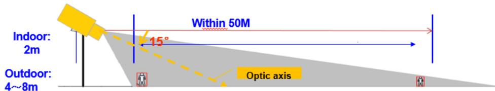
Camera is recommended to be installed 2-3 meters high in doors. If it is installed outside, it should be 3-8m high. If there is fence, the installation height must be higher than the fence.
