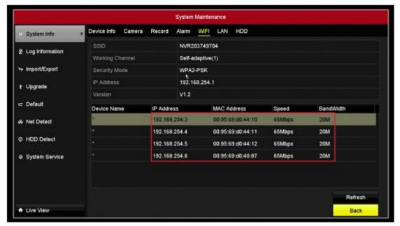
(3) If IP camera connects to the wireless of NVR successfully, NVR will automatically add IP camera with wired IP firstly. If the IP camera's password is the same as NVR's password, this step will be finished automatically.
