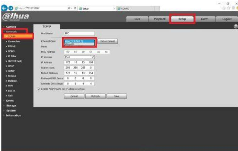
6. Select DHCP, or Configure the IP address to match the Default Gateway and Subnet mask configured in step 4, then enter in an IP within the DHCP range. For this example we will use our designated IP address from step 3 (11.1.1.108). Then select Save.
