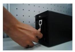
4Put the knob back after you insert the HDD to the SATA board.
