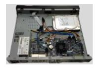
2 Place the HDD in accordance with the four holes in the bottom.
