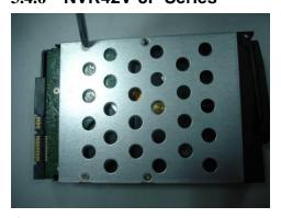
①Use 4 screws to secure the HDD
