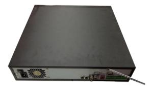
① ①Use the screwdriver to loose the screws of the rear panel and then remove the front cover.
