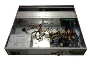
③ Connect to the HDD data cable to the main board and the HDD port respectively. Loosen the power cable of the chassis and connect another end of the power cable to the HDD port.
