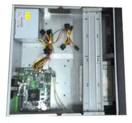
Put the bracket back. Please adjust the CD-ROM to the proper position so that the button of the front panel is directly facing the pop-up button of the CD-ROM.
