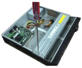
① Open top cover and then remove the ② Take off the bottom of the HDD bracket and CD-ROM HDD bracket
