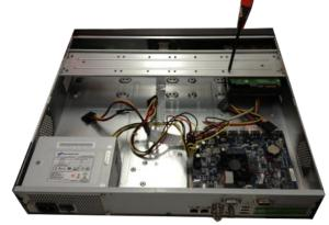
① Use the screwdriver to loose the screws of the rear panel and then remove the front cover.
